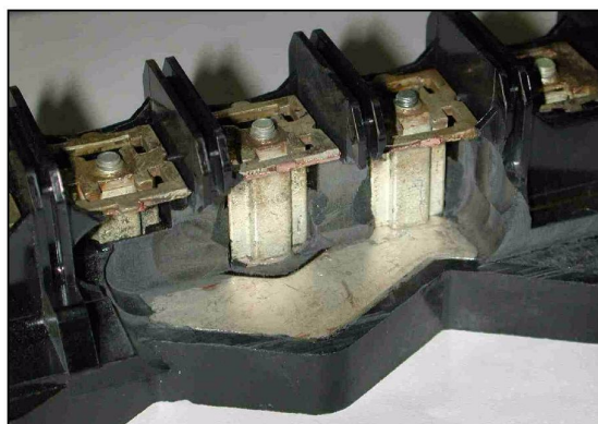
FIGURE 4 - CONDUCTING PATH FROM BUSSBAR TO STAB SOCKET
