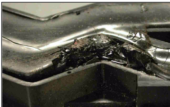
FIGURE 3 - OVERHEATING AT THE CONTACT BETWEEN THE BUSSBAR AND THE STAB SOCKET ASSEMBLY CAUSED THIS DAMAGE TO THE INSULATION. (This view is of the backside of the panel. The damage cannot be seen unless the panel is taken out of the enclosure.)
