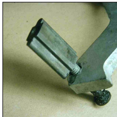
FIGURE 4 - CONDUCTING PATH FROM BUSSBAR TO STAB SOCKET
