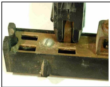
A. Copper buss bar with punched openings.
